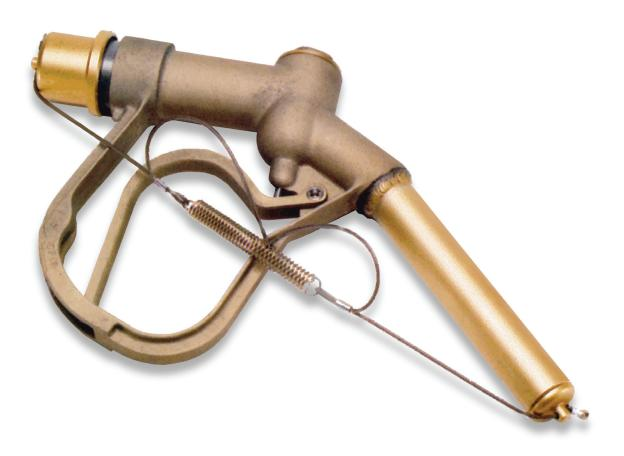
Eaton's Carter product line includes two versions of the Gravity Filling Adapter (GFA) for use with Closed Circuit Refueling nozzles (CCRs). Model 64014 (per MIL-N-52748) is for standard temperature applications. Model 64033 (per MIL-N-53093), is for arctic temperature use. The two units vary only in color (tan—standard, green—arctic) and the presence of a special, over-the-top, "arctic glove" capable operating handle on Model 64033.
