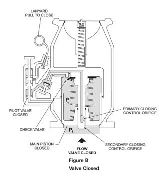
pilot valve. When it is pulled upward, the spring loaded latch attached to the lanvard pivots to lock the pilot into the open position.
