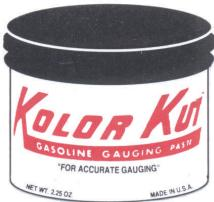
Kolor Kut Fuel Finding (Ullage) paste is light pink in colour and turns deep red upon contact with most hydrocarbon fuels. It give a clear level reading on the dip rod or tape, even when evaporation at the interface would normally cause distortion of the reading. Kolor Kut Fuel Finding Paste is supplied in 2.25 oz. tubs only.
